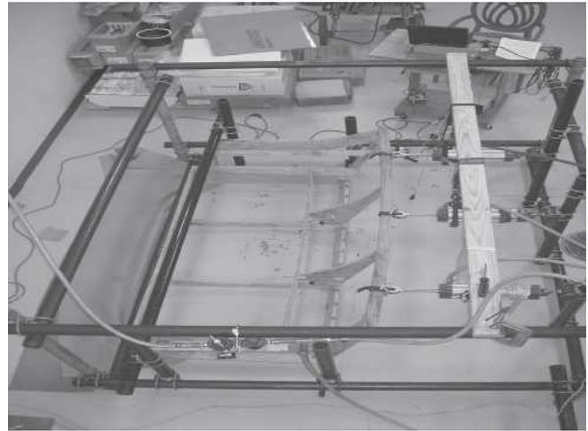
Figure 3. — Set-up for the sofa backrest frame test.
