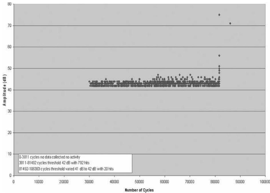
Figure 6. — A typical example of AE hit data (Amplitude vs. Number of cycles) collected by the acoustic emission measuring system through the microphone as noise detecting sensor.
