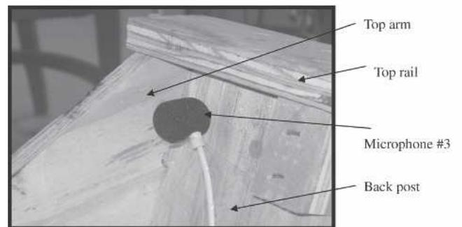
Figure 5. — Location of microphones #1, #2, and #3 for the backrest frame test.
