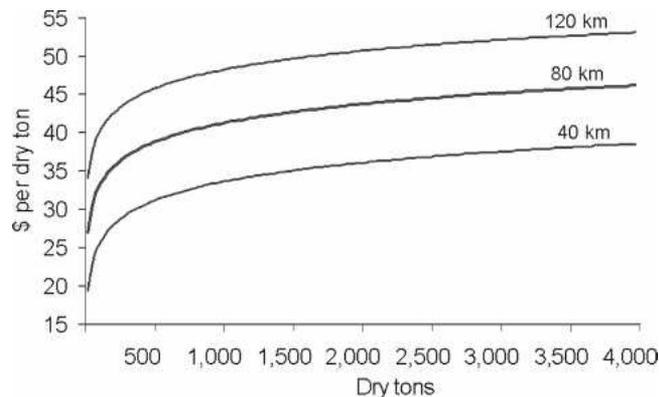
Figure 1. — Adjusted cost curves of woody biomass feedstocks for three procurement distances in Mississippi (Source: Grebner et al. In press).
