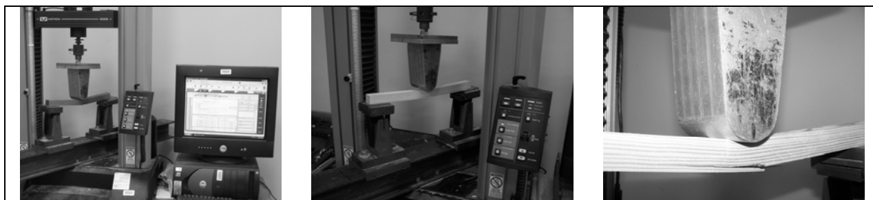
Figure 2. Typical bending test set-up
