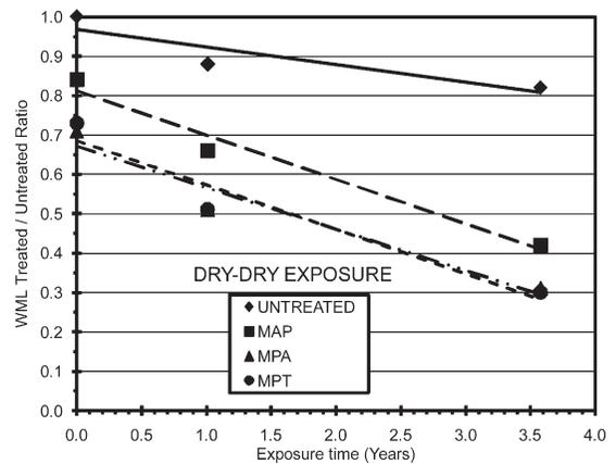
Figure 8. Ratio of treated/untreated WML for samples exposed in the DRY-DRY condition.
