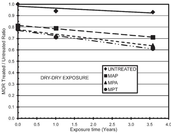
Figure 5. Ratio of treated/untreated MOR for samples exposed in the DRY-DRY condition.
