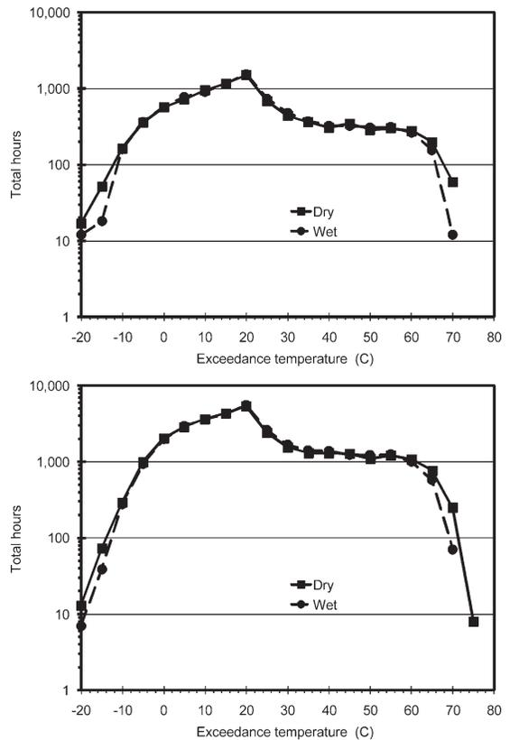
Figure 3. Temperature loads during the 1-yr (upper) and the 3.6-yr (lower) exposure periods.
