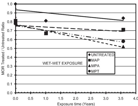
Figure 7. Ratio of treated/untreated MOR for wet samples exposed under wet conditions.
