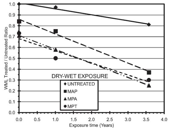
Figure 9. Treated/untreated WML ratio for samples exposed under DRY-WET conditions.
