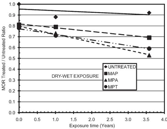
Figure 6. Treated/untreated MOR ratio for samples exposed under DRY-WET conditions.
