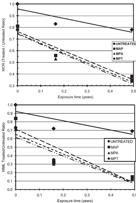
Figure 4. Comparison of treated/untreated MOR (upper) and WML (lower) ratios in the laboratory study.
