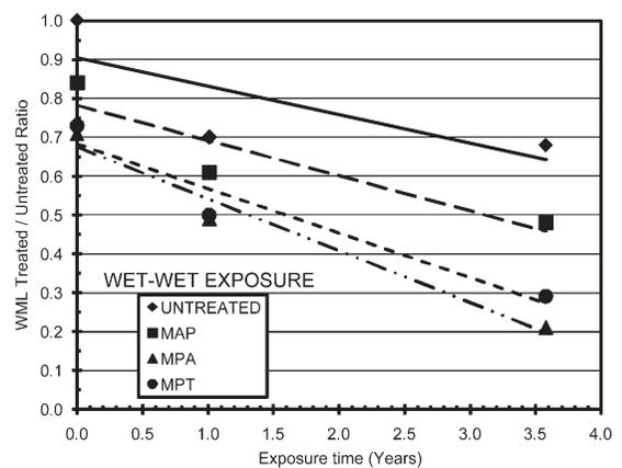
Figure 10. Ratio of treated/untreated WML for wet samples exposed under wet conditions.
