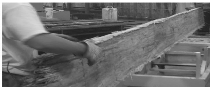
*Figure 1. Typical rough beam shown immediately after pressing.*
