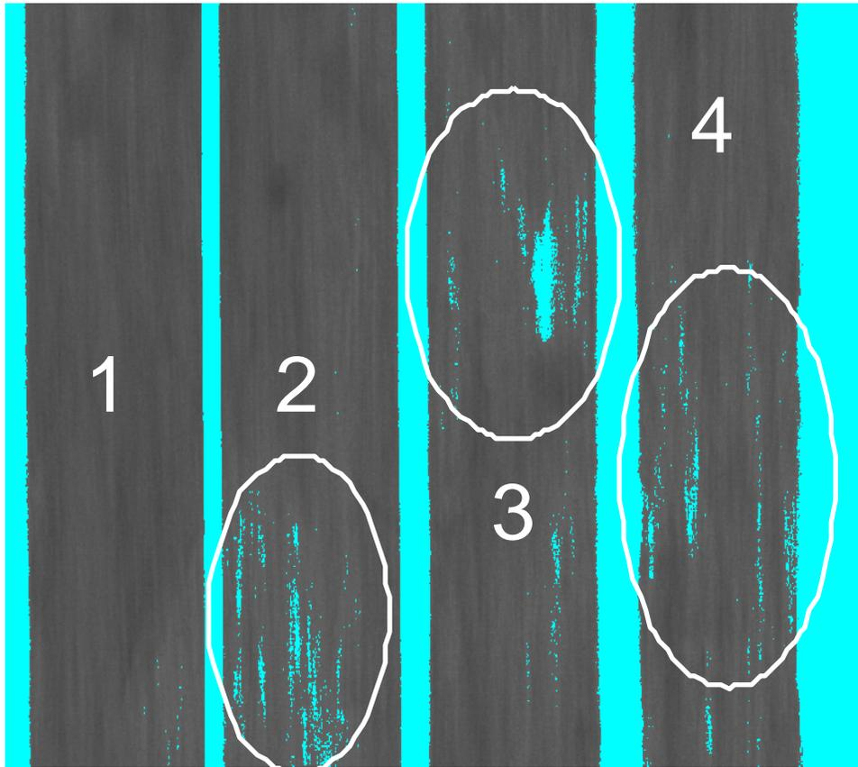
*Figure 3. X-ray images of SPSL beams showing areas of low density (denote by circles).*
