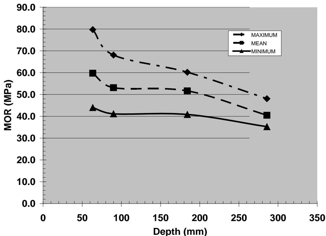
*Figure 3: MOR depth effects for beams tested in static bending.*
