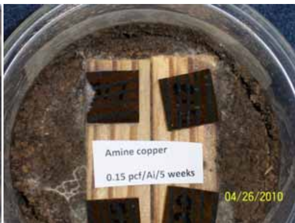
Figure 3 (right) and Figure 4 (left). Notice the minimal fungal mycelia growing on the top of both wafers at the lowest treatment level examined of amine soluble copper of 0.15 pcf, compared to the heavy mycelium at the highest treatment level of 0.30 pcf with particulate copper in Figures 1 and 2.
