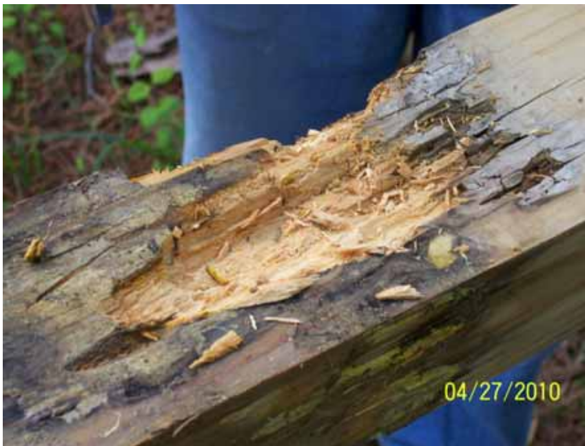
Figure 14. A typical MCA-treated 4x4 post after 11 months of exposure in the accelerated plot. Note the extensive decay on the top face, and the decay on the next face. All four faces are rated separately, and then the average of all four faces or the rating of the worse face were reported.
