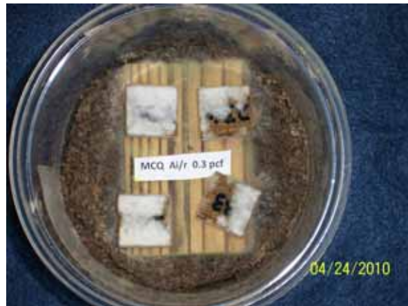
Figures 7 (left) and 8 (right). Pictures show wood treated with MCQ to 0.30 pcf after 9 weeks of incubation to two copper-tolerant fungi. Note the relative heavy fungal mycelia growth on the tops of the treated wafers.
