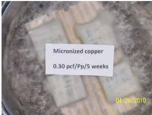
Figure 1 (left) and Figure 2 (right). Notice the heavy mycelia growth of both copper-tolerant fungi on top of the particulate copper-treated wafers even at the highest treatment level of 0.30 pcf. The fungus on the right was a gift from the USDA-Forest Products Laboratory. It was identified as A. incrassata when first isolated from the Harrison National Forest near the Gulf Coast of Mississippi and was later re-identified as Antrodia radiculosa .
