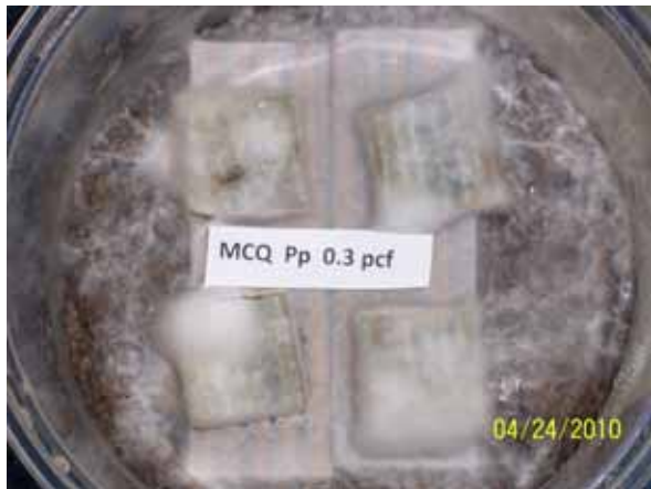
Figures 7 (left) and 8 (right). Pictures show wood treated with MCQ to 0.30 pcf after 9 weeks of incubation to two copper-tolerant fungi. Note the relative heavy fungal mycelia growth on the tops of the treated wafers.
