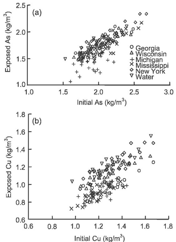
FIG. 1. Final versus initial biocide retention per specimen for As (a) and Cu (b).
