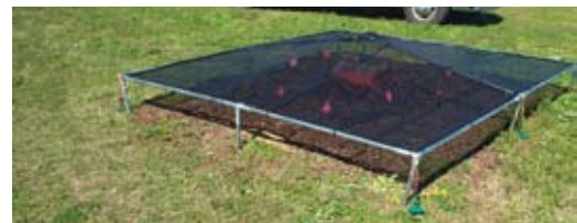
Figure 2 - Post-beam structures have been constructed over transplanted FST colonies for future testing of building materials (above). Small-scale field testing with FST is also being investigated (below).
