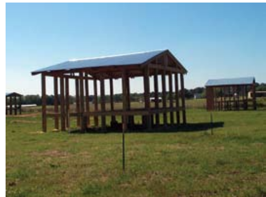
Figure 2 - Post-beam structures have been constructed over transplanted FST colonies for future testing of building materials (above). Small-scale field testing with FST is also being investigated (below).
