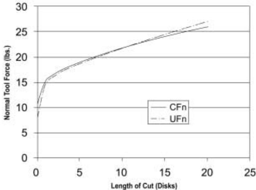
Figure 1. — The fitted non-linear normal force regression curves for the cryogenic-treated ( $CF_n$ ) and untreated ( $UF_n$ ) tungsten carbide with 10-degree clearance and 15-degree rake angle, respectively.
