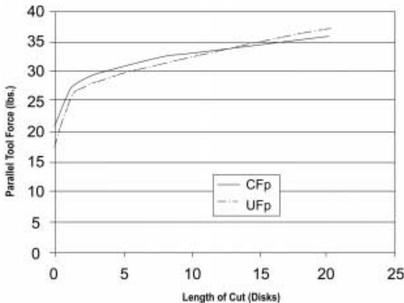
Figure 2. — The fitted non-linear parallel force regression curves for the cryogenic-treated ( $CF_p$ ) and untreated ( $UF_p$ ) tungsten carbide with 10-degree clearance and 15-degree rake angles, respectively.
