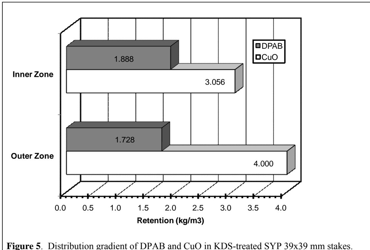
**Figure 5.** Distribution gradient of DPAB and CuO in KDS-treated SYP 39x39 mm stakes.
