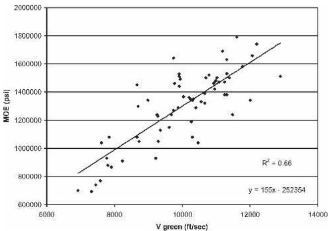
Figure 1. — Plot of acoustic velocity (green) vs. MOE.
