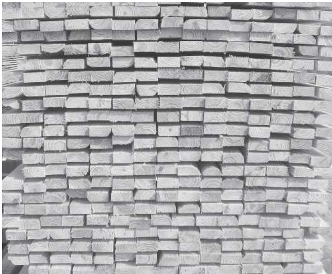
Figure 2. — Photograph of green 2 by 4 lumber sawn from small-diameter loblolly pine thinnings (photo courtesy D.L. Buckner).
