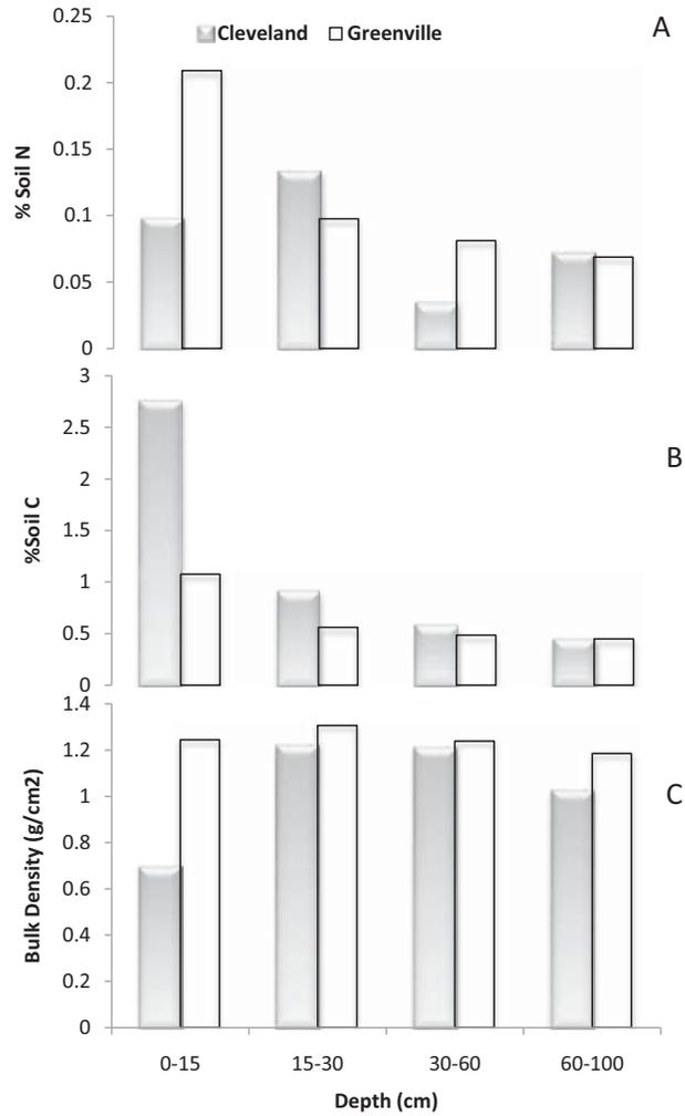
Figure 2—Changes in soil properties with depth: (A) mean amount soil N, (B) mean amount soil C, and (C) bulk density of the soil with depth on two former agricultural sites at the LMAV.
