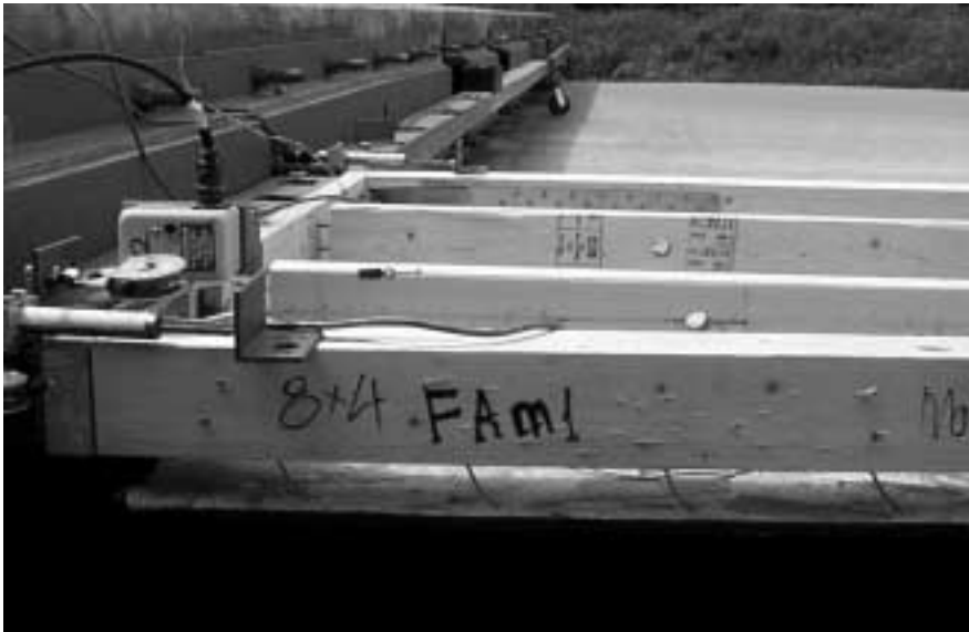
Figure 11. — Typical failure mode of walls with low-density end studs.
