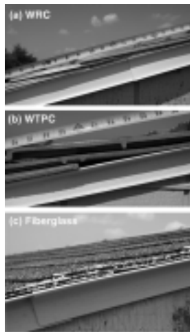
Figure 2. — Side view of shingles installed in 2001 at Valley View test site in Wisconsin. Ruler shown in inches.
