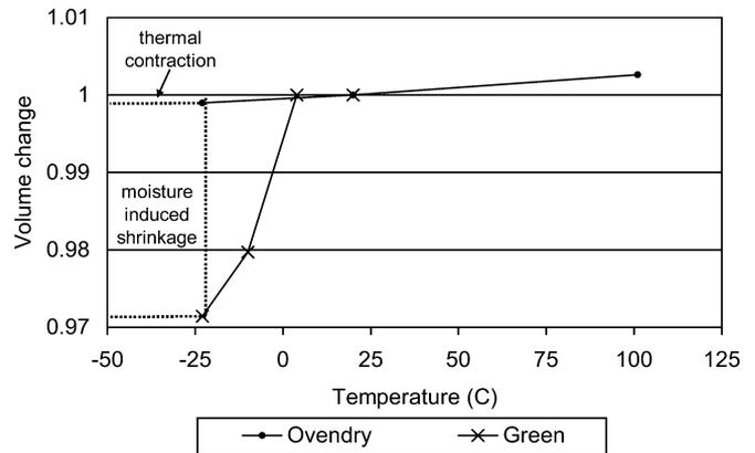
**Figure 2.** — Graphical presentation of volumetric shrinkage for oven-dry and wetwood by temperature. Volume data points are standardized such that 4°C equals unity.
