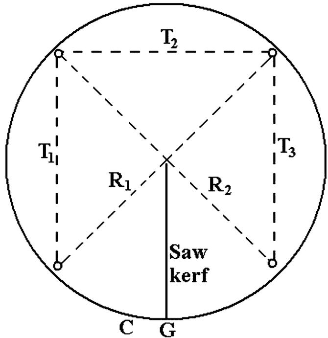
Figure 1. — Illustration of the three tangential ( $T_n$ ), two radial ( $R_n$ ), circumferential (C), and gap (G) measurement lines per disk.
