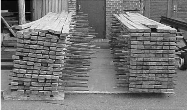
Figure 4. — Photograph of nonrestrained control (left) and restrained (right) lumber packages shortly after removal from the kiln and the restraint device.
