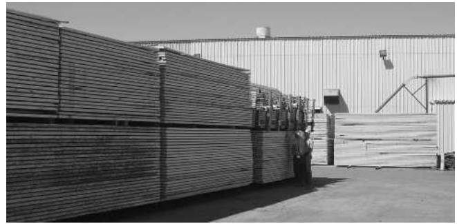
Figure 2. — Restraint lumber package incorporated in full kiln charge readied for drying.
