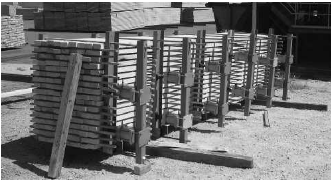
Figure 1. — Restraint device secured on test lumber package.
