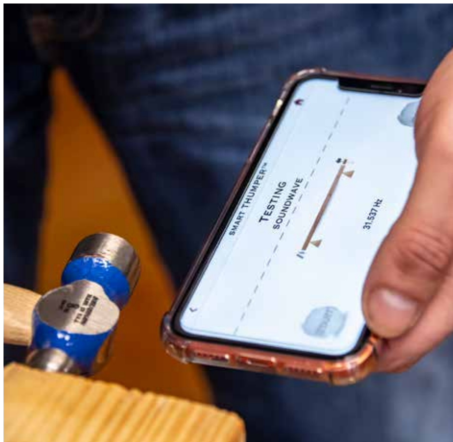
The Smart Thumper app uses sound or vibration to evaluate lumber. (Photo by David Ammon)
