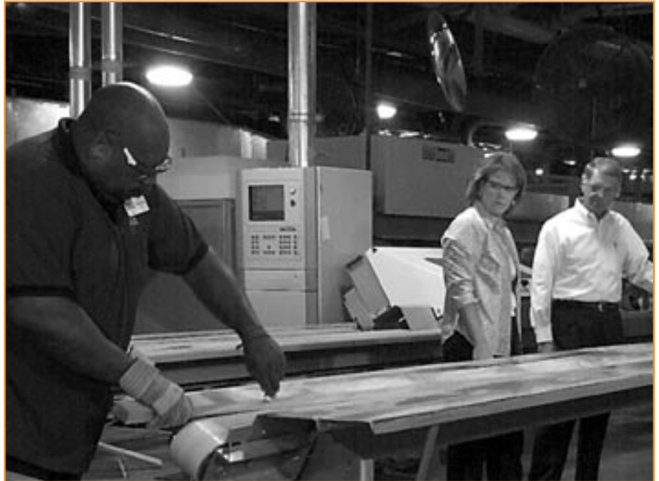
Airline Manufacturing Company president Judy Dunaway (center) and Duane Motsenbocker (r) watch an employee mark defects between interconnected CNC rip and crosscut saws.
